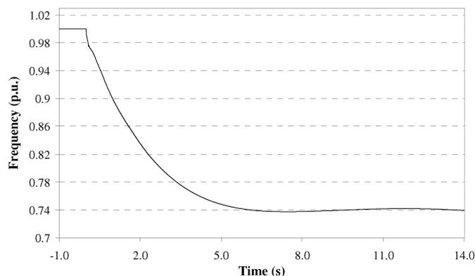
Fig. 11. System frequency during islanding and nonoptimal load shedding for case 2.
