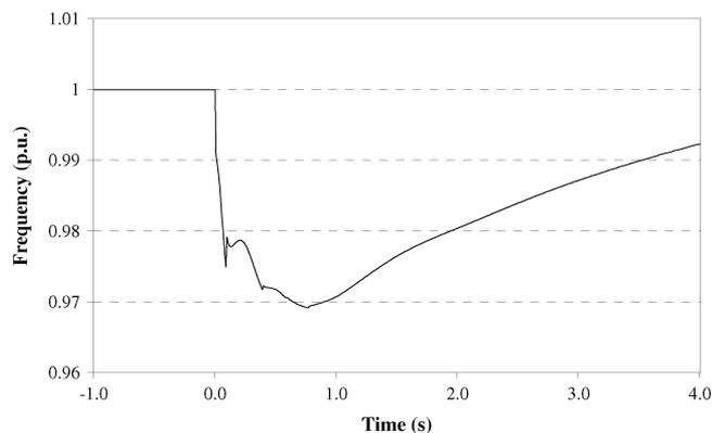
Fig. 8. System frequency during islanding and load shedding for case 3.
