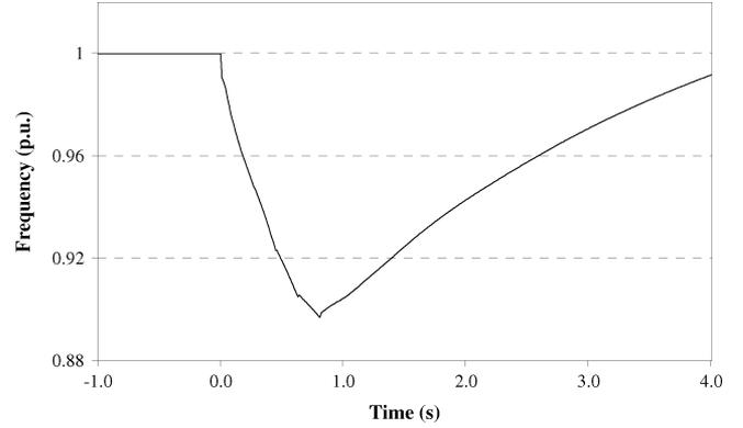
Fig. 4. System frequency during islanding and load shedding for case 1.
