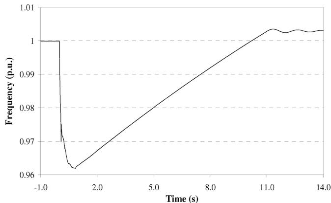
Fig. 13. System frequency during islanding and load shedding for case 4.
