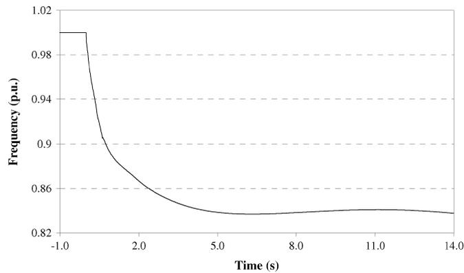
Fig. 10. System frequency during islanding and nonoptimal load shedding for case 1.
