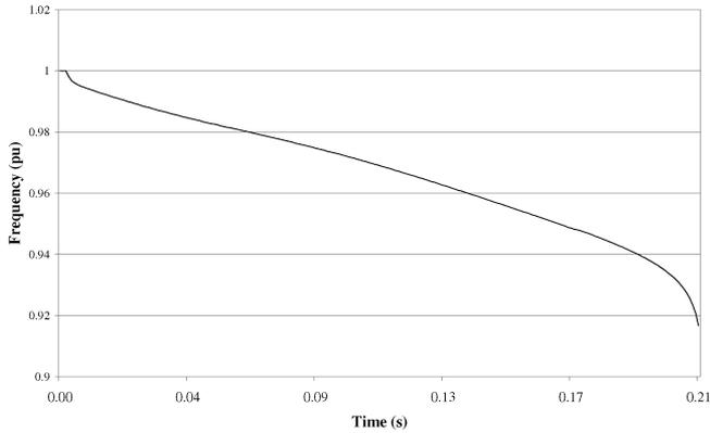
Fig. 1. System frequency after islanding.
