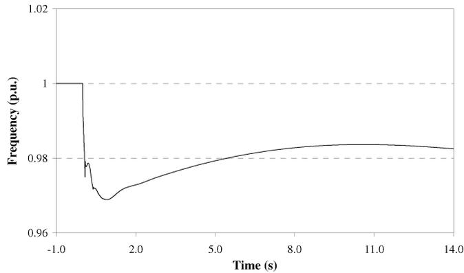
Fig. 12. System frequency during islanding and nonoptimal load shedding for case 3.
