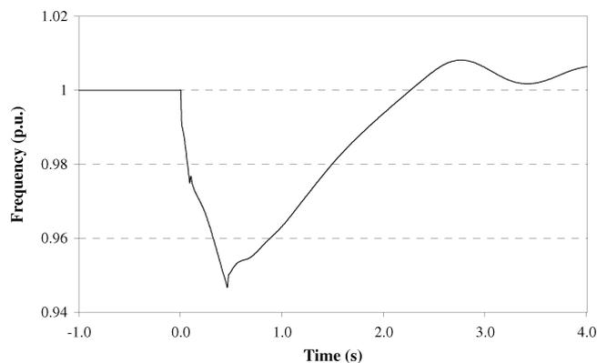
Fig. 6. System frequency during islanding and load shedding for case 2.
