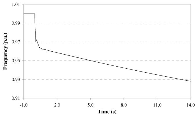
Fig. 14. System frequency during islanding and nonoptimal load shedding for case 4.
