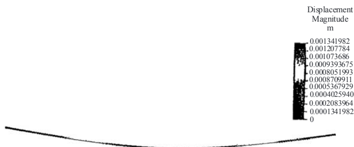
Figure 1 : 400mm beam deflection with shear area included
