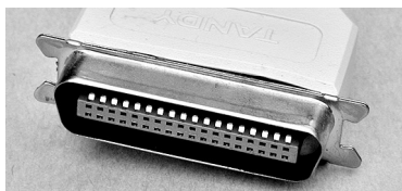
FIGURE 54. Centronics interface connector
