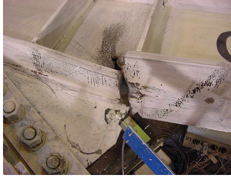
Fig. 15 Fracture in Beam at End of Gusset Plate, 2.6% Drift, Test No. 3
